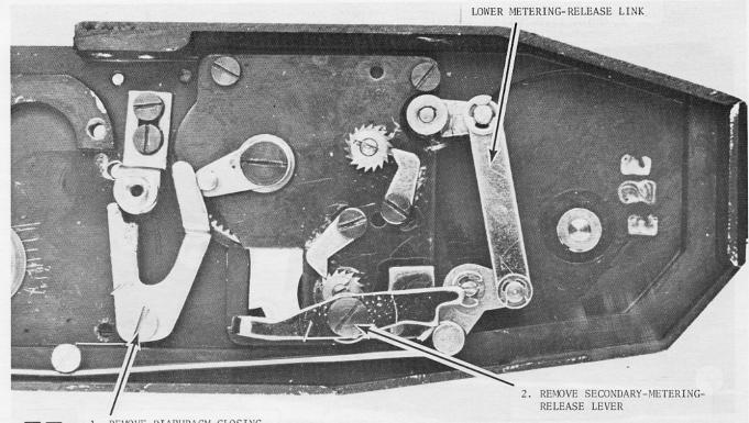
1. REMOVE DIAPHRAGM-CLOSING-LEVER LATCH
