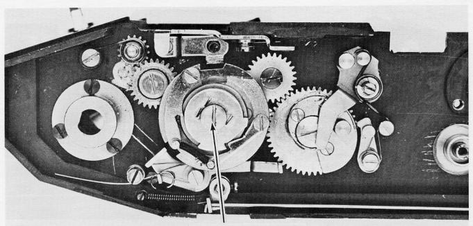
REMOVE SCREW AND LIFT OFF OPENING-CURTAIN CAM
