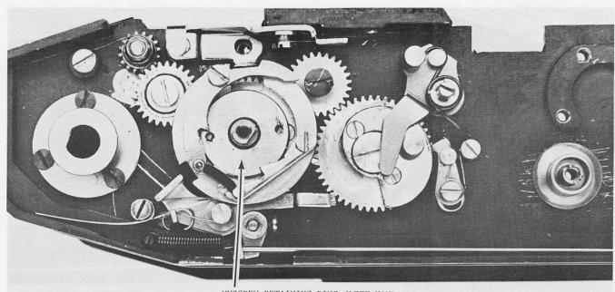
UNSCREW RETAINING RING (LEFT-HAND THREAD) AND LIFT OFF MAIN-TRANSPORT CAM
